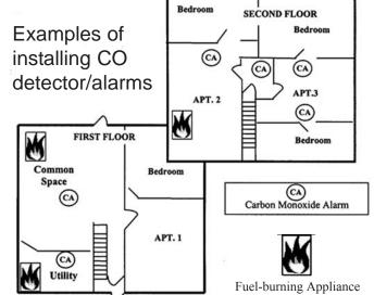
\*An exception to installation of CO detector/alarms: If the building is pre-October 2008, CO detector/alarms are not needed if there is no enclosed attached garage and all fuel-burning devices are closed-combustion (do not release combustion air to the interior of the building). Those closed-combustion devices require annual inspections.
