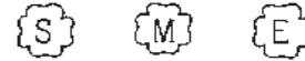
FIG. PG-105.1 OFFICIAL SYMBOLS FOR STAMPS TO DENOTE THE AMERICAN SOCIETY OF MECHANICAL ENGINEERS' STANDARD FOR BOILERS
