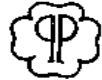
FIG. PG-105.3 OFFICIAL SYMBOL FOR STAMP TO DENOTE THE AMERICAN SOCIETY OF MECHANICAL ENGINEERS' STANDARD FOR WELDED PIPING
