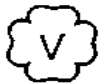
FIG. PG-105.4 OFFICIAL SYMBOL FOR STAMP TO DENOTE THE AMERICAN SOCIETY OF MECHANICAL ENGINEERS' STANDARD
