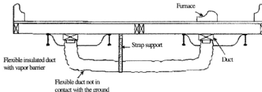
Notes: 1. This system is typically used when a crossover duct has not been built into the floor and the furnace is situated directly over the main duct in one section of the home. A single flexible duct is then used to connect the two sections to each other.
