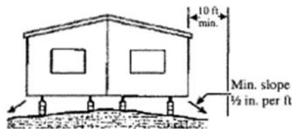
Home sites must be prepared so that there will be no depressions in which surface water may accumulate beneath the home. The area of the site covered by the manufactured home must be graded, sloped, or designed to provide drainage from beneath the home or to the property line
