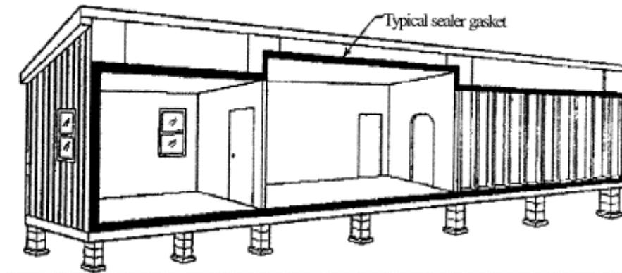
Note: On multi-section manufactured homes, install the sealer gasket on the ceiling, end walls, and floor mate-line prior to joining the sections together.
