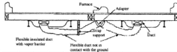
Notes: 1. This system is typically used when a crossover duct has not been built into the floor and the furnace is outside the I-Beam. With this type of installation, it is necessary for two flexible ducts to be installed.
