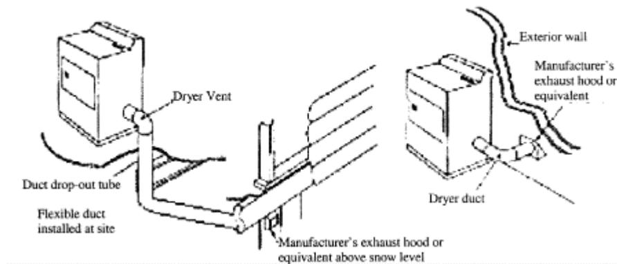
Notes: 1. Installation of the exhaust system must be in accordance with the dryer manufacturer instructions.
