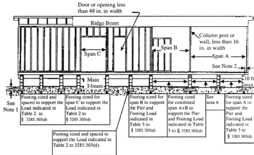
Notes: 1. Bottom of footings must be below the frost line depth, unless designed for placement above the frost line. (See §3285.312(b)).
