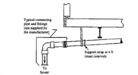
Note: Fittings in the drainage system that are subject to freezing, such as P-traps in the floor, are protected with insulation by the manufacturer. Insulation must be replaced if it is removed for access to the P-trap.
