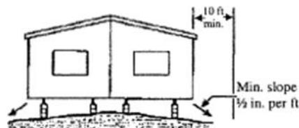
Home sites must be prepared so that there will be no depressions in which surface water may accumulate beneath the home. The area of the site covered by the manufactured home must be graded, sloped, or designed to provide drainage from beneath the home or to the property line
