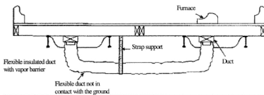
Notes: 1. This system is typically used when a crossover duct has not been built into the floor and the furnace is situated directly over the main duct in one section of the home. A single flexible duct is then used to connect the two sections to each other.
