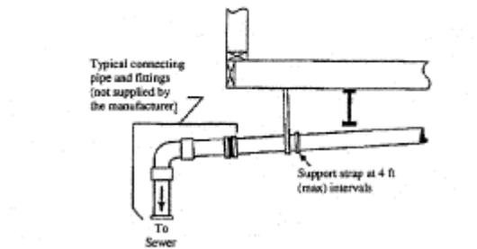
Note: Fittings in the drainage system that are subject to freezing, such as P-traps in the floor, are protected with insulation by the manufacturer. Insulation must be replaced if it is removed for access to the P-trap.
