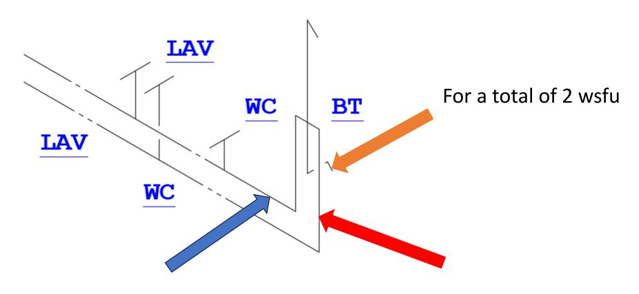
Assign 1.5 wsfu (1.5 gpm) to each side =  $\frac{1}{2}$ " diameter piping for each fixture supply
