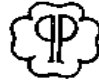
FIG. PG-105.3 OFFICIAL SYMBOL FOR STAMP TO DENOTE THE AMERICAN SOCIETY OF MECHANICAL ENGINEERS' STANDARD FOR WELDED PIPING
