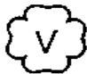
FIG. PG-105.4 OFFICIAL SYMBOL FOR STAMP TO DENOTE THE AMERICAN SOCIETY OF MECHANICAL ENGINEERS' STANDARD
