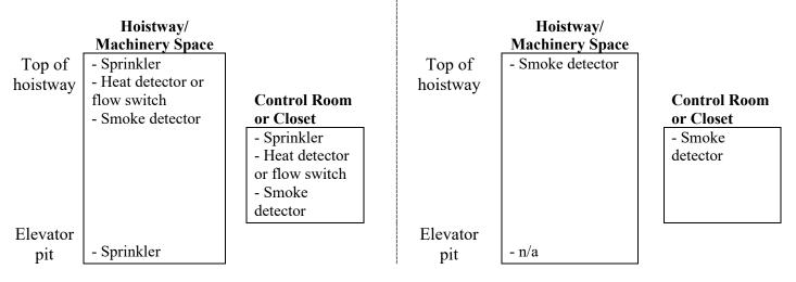
Case 4b-2: Building completely sprinklered per NFPA 13.
