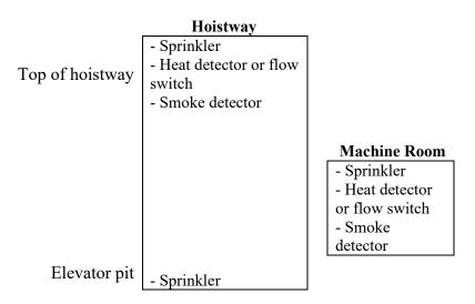
Case 9: Building partially sprinklered per NFPA 13R.
