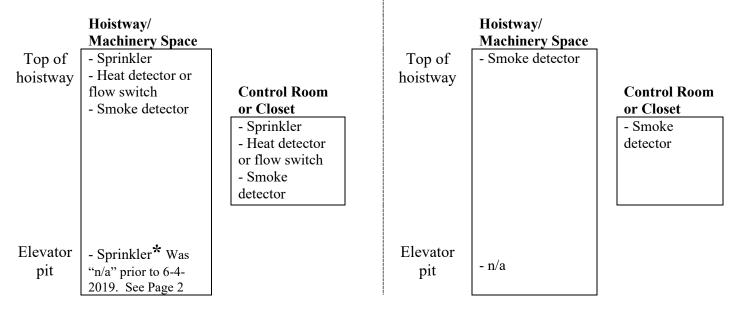
**<u>Case 4c:</u>** Building completely sprinklered per NFPA 13.
