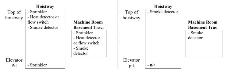
**<u>Case 1b:</u>** Building completely sprinklered per NFPA 13.
