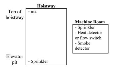
Case 2a: Building completely sprinklered per NFPA 13.
