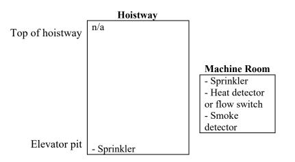
Case 9a: Building partially sprinklered per NFPA 13R.
