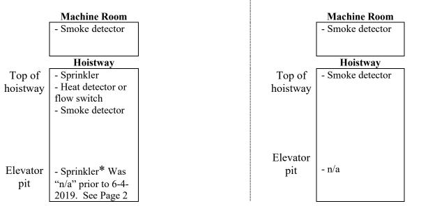
**<u>Case 11:</u>** Building partially sprinklered per NFPA 13R.
