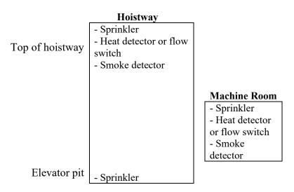
Case 10: Building partially sprinklered per NFPA 13R.
