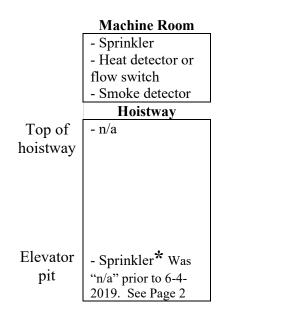
Building Code Applies Date On or After May 1, 2018 with FT-1 Rated Suspension Means
