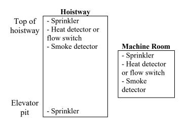
**<u>Case 3:</u>** Building completely sprinklered per NFPA 13.
