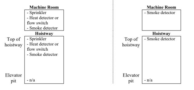
**<u>Case 4b-1</u>**: Building completely sprinklered per NFPA 13.
