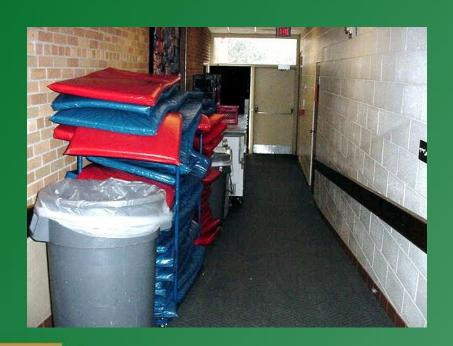
10.19.5.1 Combustible material shall not be stored in boiler rooms, mechanical rooms, or electrical equipment rooms.
