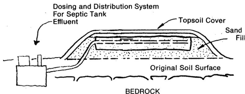
In an existing mound, careful dosing and distribution are essential to proper purification of the septic tank effluent. Air spaces are also important.
