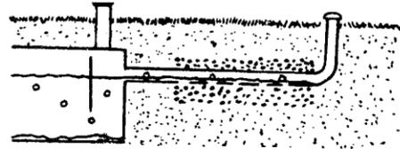
Viruses and bacteria get free from the solids, and proceed out the effluent pipe to the soil absorption system. The soil can only stop these biologic contaminants if the soil layer is deep enough, and if the effluent passes through slowly enough.
