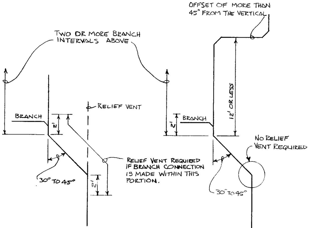
A-82.31 (5) (b) RELIEF AND YOKE VENTS FOR OFFSETS OF MORE THAN 45 DEGREES.
