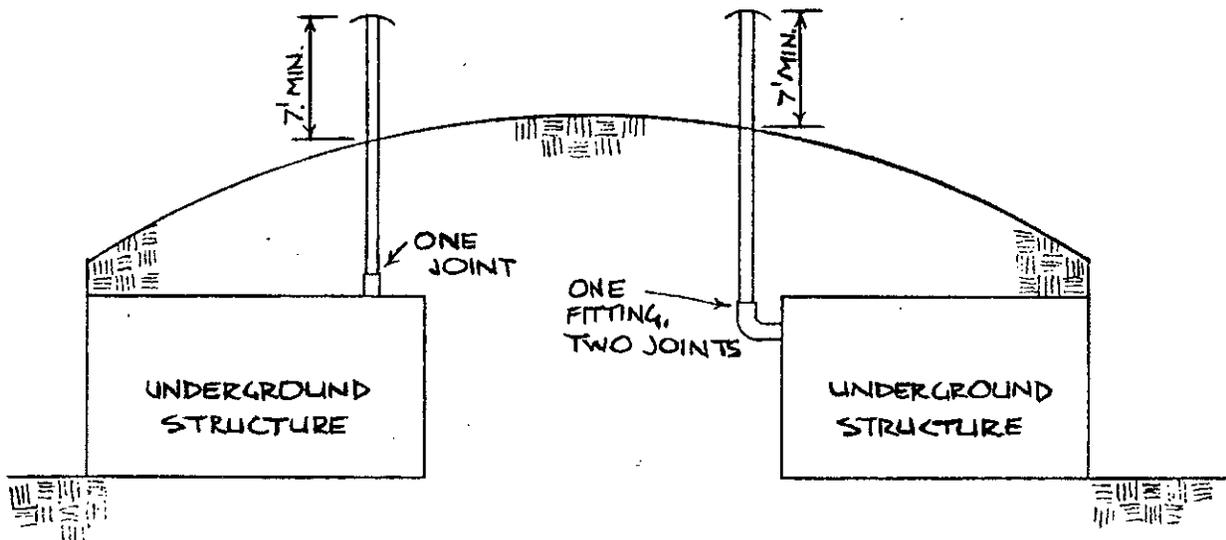
VENT TERMINALS FOR UNDERGROUND STRUCTURES
