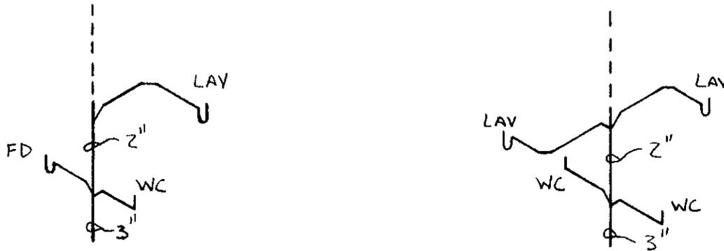
COMMON VENT FOR FLOOR OUTLET FIXTURES
