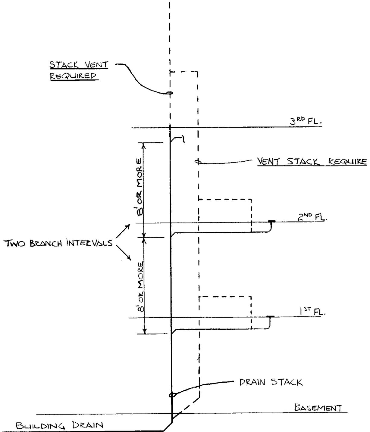
A-82.31 (4) (a) WHERE A VENT STACK AND STACK VENT ARE NOT REQUIRED.
