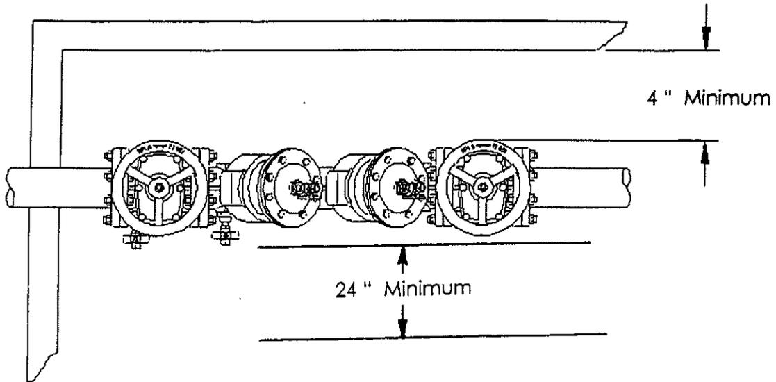
NOTE: ASSEMBLIES SHALL BE INSTALLED IN ACCORDANCE WITH THE MANUFACTURER'S WRITTEN INSTALLATION SPECIFICATIONS OR WITHIN THE DIMENSIONS SHOWN.
