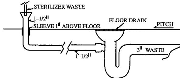
3. Battery assemblies. A battery assembly of not more than 3 sterilizer wastes may drain to one trap, provided the trap and waste are sized according to the combined fixture unit rating; the trap is located immediately below one of the indirect waste connections; the developed distance of a branch does not exceed 8 feet; and the branches change direction through a tee-wye or wye pattern fitting.
