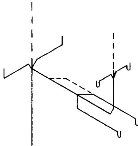
A-82.31 (13) (c) WET VENTING - FLOOR OUTLET FIXTURES.
