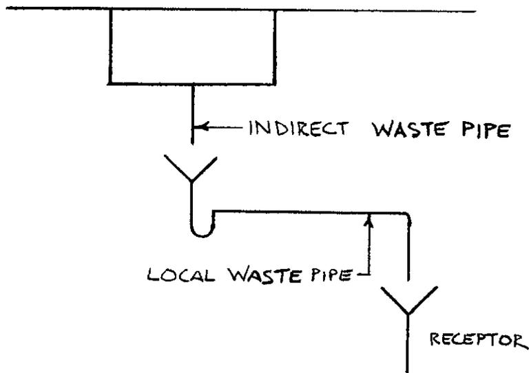
A-82.33 (8) (a) WASTE SINKS AND STANDPIPES.
