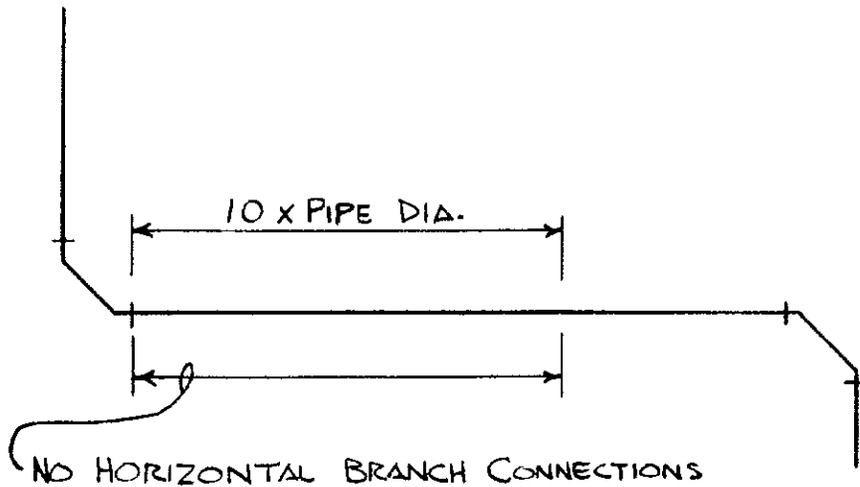
A-82.30 (7) HORIZONTAL BRANCH DRAIN CONNECTION AT BASE OF A STACK.
