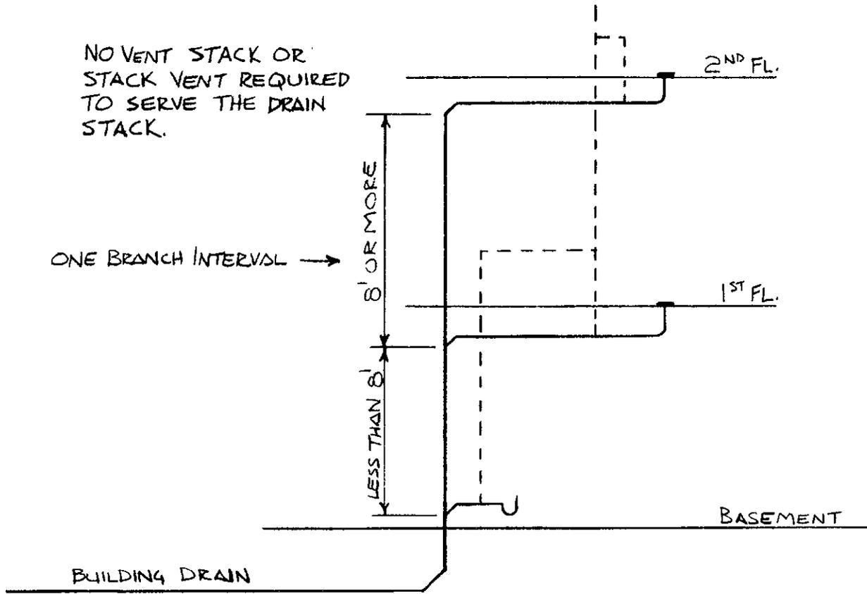
A-82.31 (4) (b) INSTALLATION OF VENT STACK AND STACK VENT.
