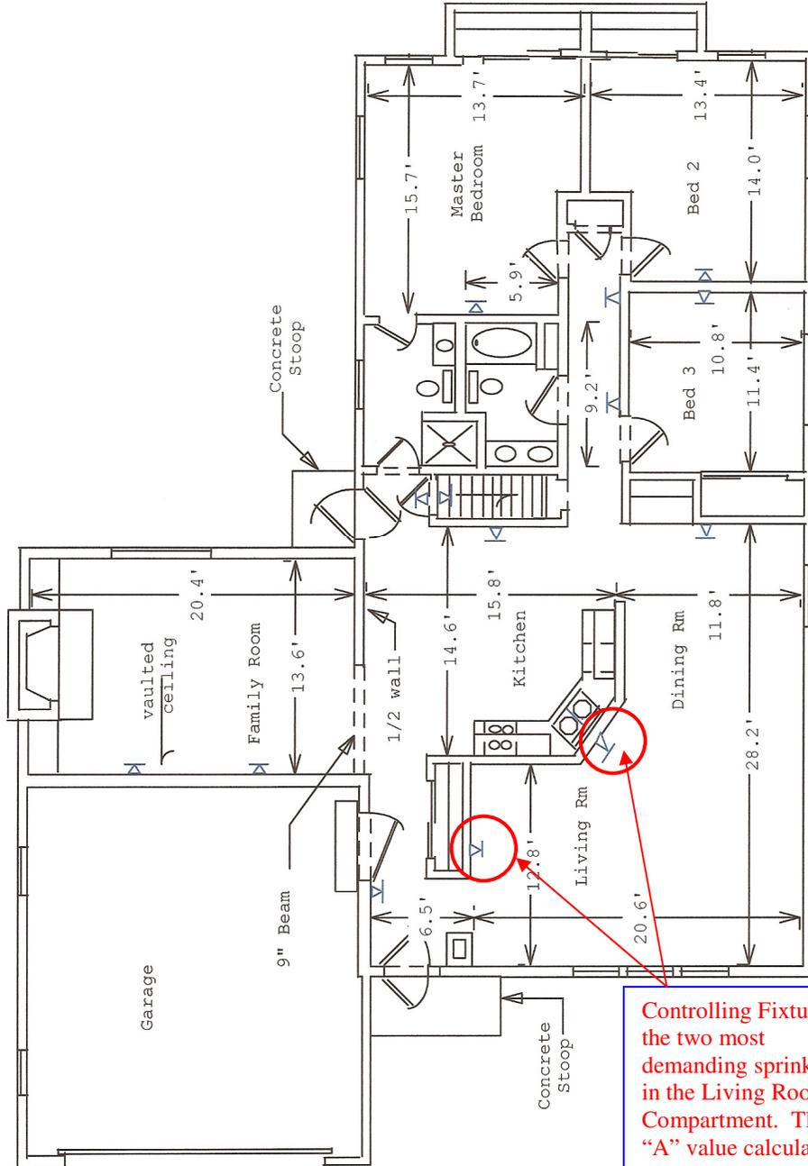
Controlling Fixture is the two most demanding sprinklers in the Living Room Compartment. The "A" value calculated will be the set value for the entire fire-water distribution system
