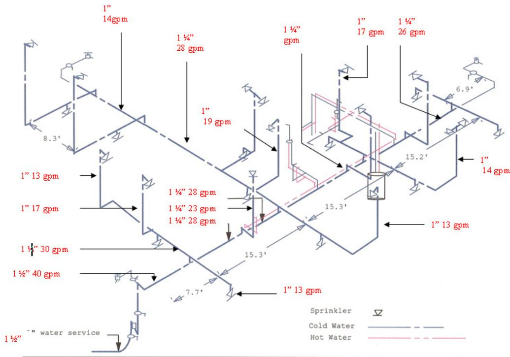
Isometric of the fire-water distribution system, with sizing gpm load requirements.
