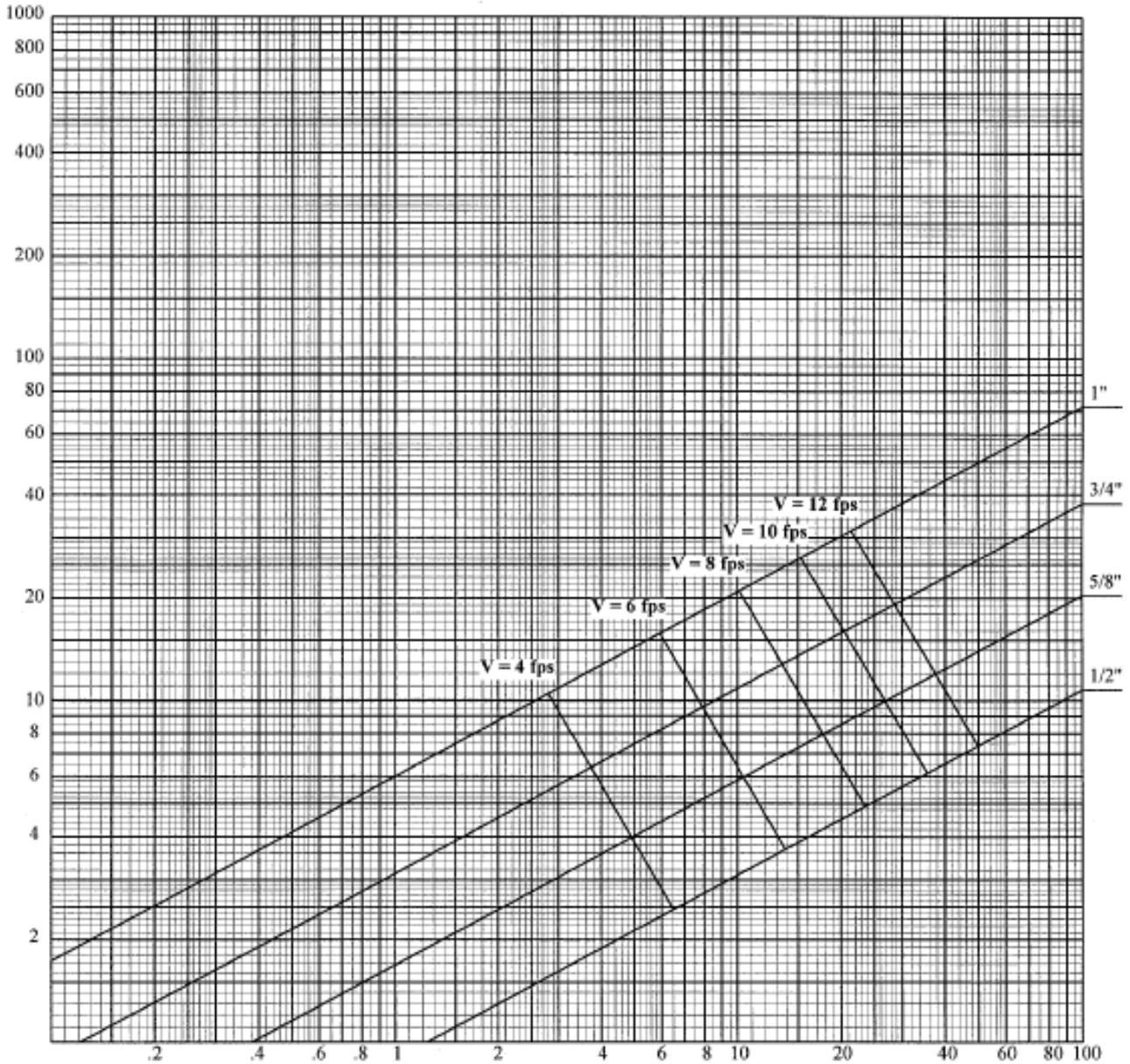
Pressure loss due to friction (psi/100 ft of pipe)
