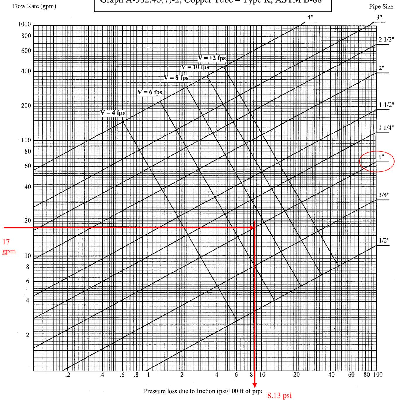
✚ The last section of the Fire – Water Calc Worksheet is provided in Figure 6-7. The final steps of B – G. will provide an “A” value which represents the available pressure for uniform loss per 100 feet. From this “A” value we will be able to refer to our material tables and size the water distribution system according to the gpm demand or load and its relationship to the pressure available to serve the sprinklers or plumbing fixtures.
