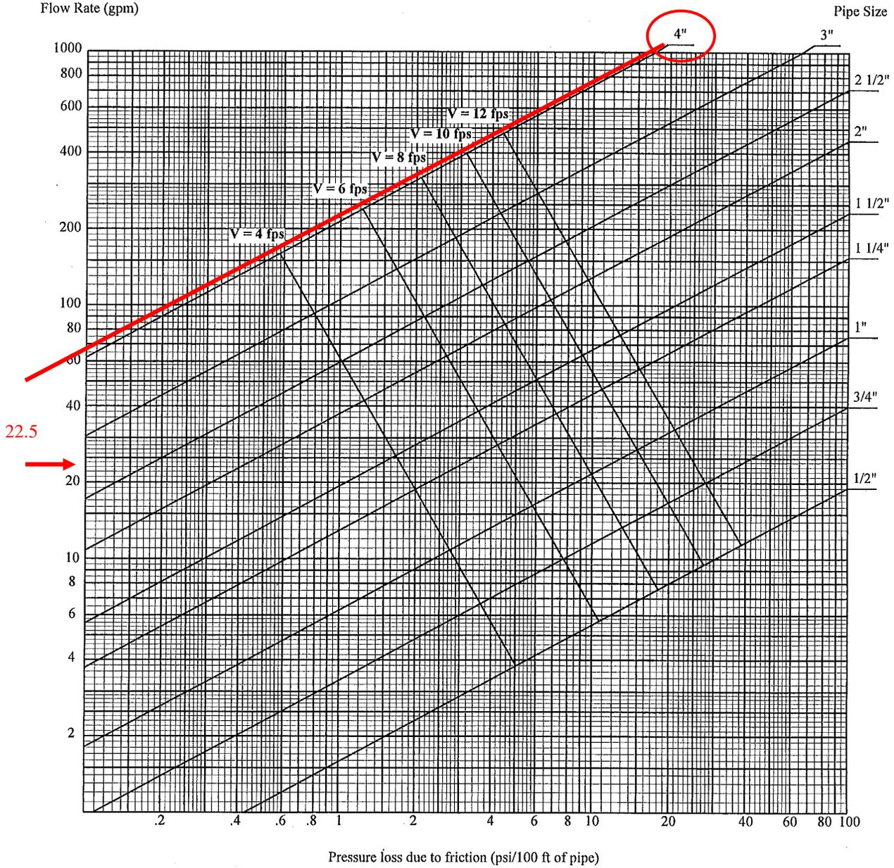
Fractional friction loss on a 4 inch water service and a 22.5 domestic water building demand.
