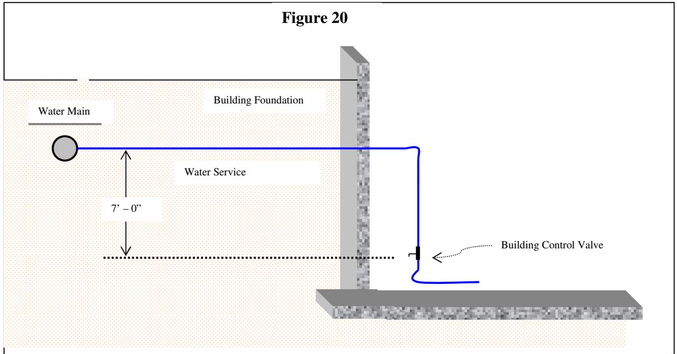
One more example: You have been contacted to install the water service piping from a water main installed at an elevation of 103 feet to a slab constructed building with a building control valve at an elevation of 117 feet. The building control valve is higher in elevation than the water service is. There will be a pressure loss through the water service piping due to this elevation difference.
