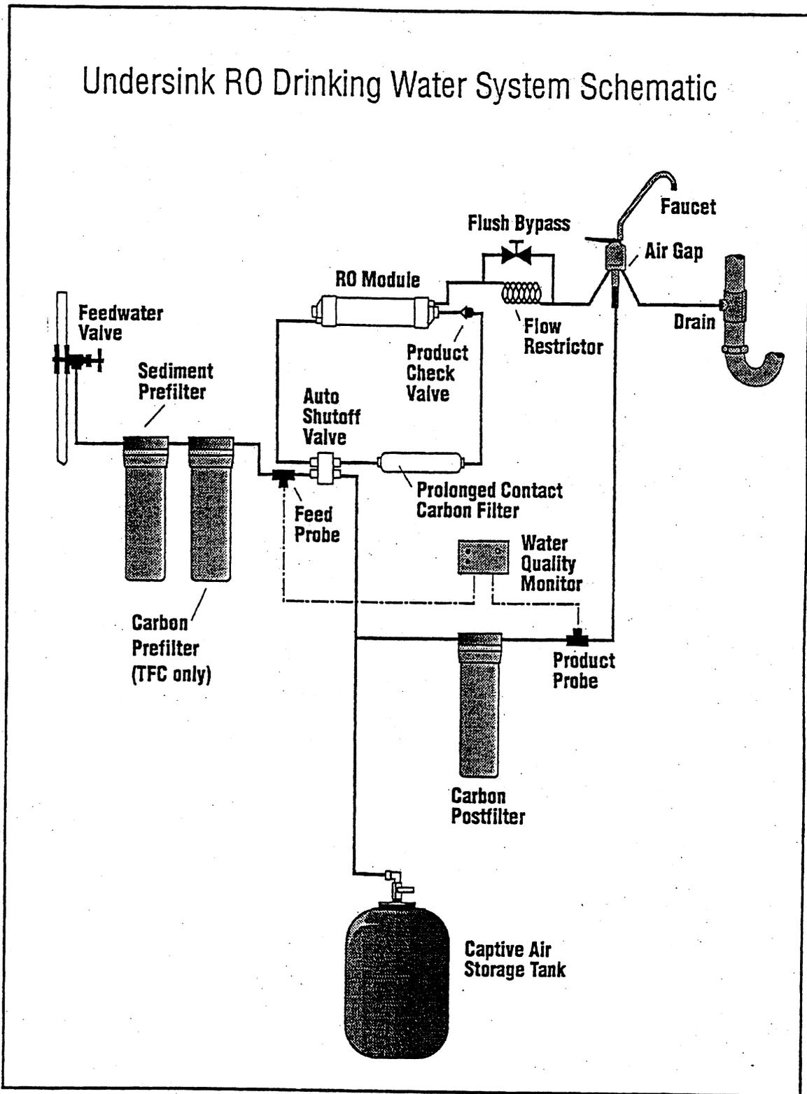
Figure 4-5: Typical under-cabinet installation
