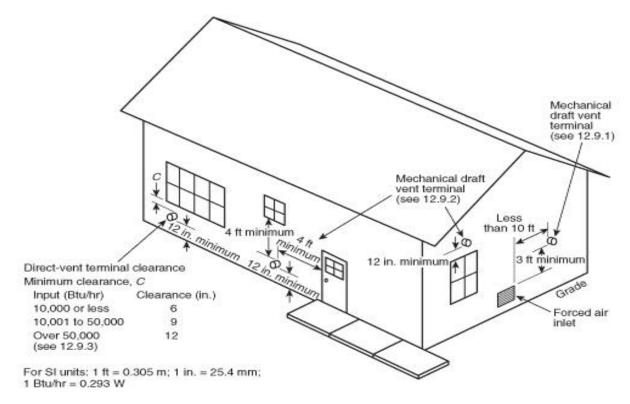
**Exit Terminals of Mechanical Draft and Direct-Vent Venting Systems.** Above diagram shows gas vent terminal clearances from the Appendix of NFPA 54 standard.
