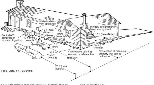
Note 1: Regardless of its size, any ASME container filled on site must be located so that the filling connection and fixed maximum liquid level gauge are at least 10 ft from any external source of ignition (e.g., open flame, window A/C, compressor), intake to direct-vented gas appliance, or intake to a mechanical ventilation system. Refer to 6.3.9.
