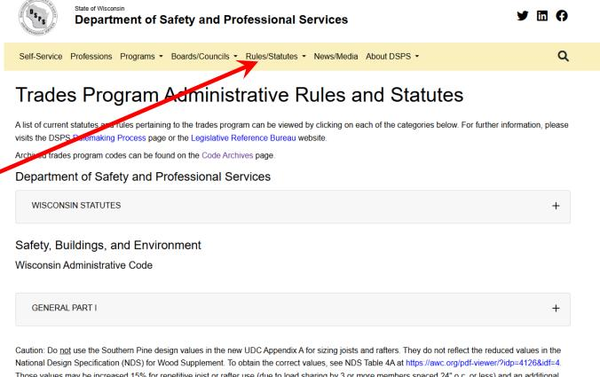
Those values may be increased 15% for repetitive joist or rafter use (due to load sharing by 3 or more members spaced 24" o.c. or less) and an additional 15% for rafter use (due to snow load duration increase).
