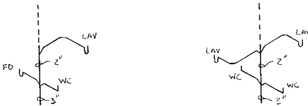
COMMON VENT FOR FLOOR OUTLET FIXTURES SERVING AS A WET VENT
