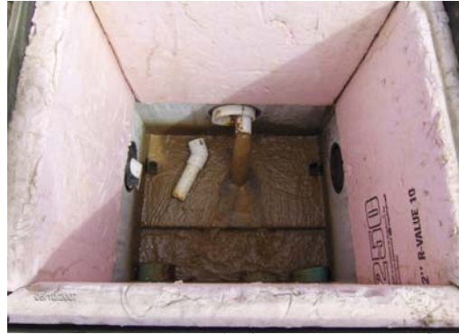
Figure 2. The four-inch underdrain is connected to a watertight bulkhead fitting. The drain pipe on the outside fitting is directed into a distribution box for sample collection.
