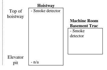
**<u>Case 1b:</u>** Building completely sprinklered per NFPA 13.
