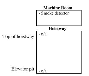
Case 8: Building partially sprinklered per NFPA 13R.
