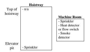
Case 2a: Building completely sprinklered per NFPA 13.
