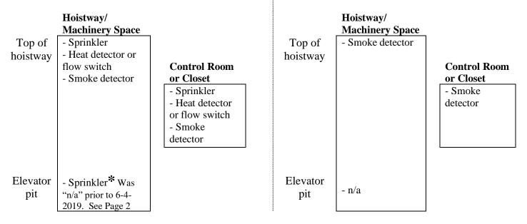
Case 4c: Building completely sprinklered per NFPA 13.
