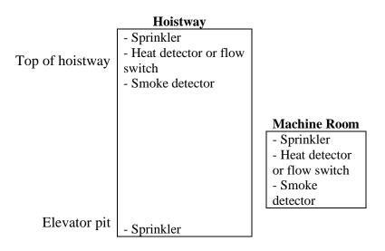
Case 10: Building partially sprinklered per NFPA 13R.
