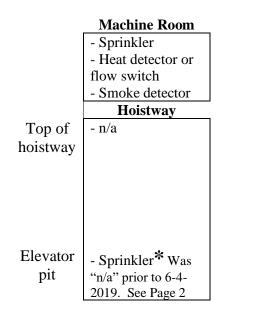
Building Code Applies Date On or After May 1, 2018 with FT-1 Rated Suspension Means
