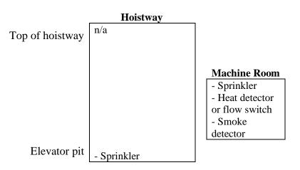
**<u>Case 9a:</u>** Building partially sprinklered per NFPA 13R.
