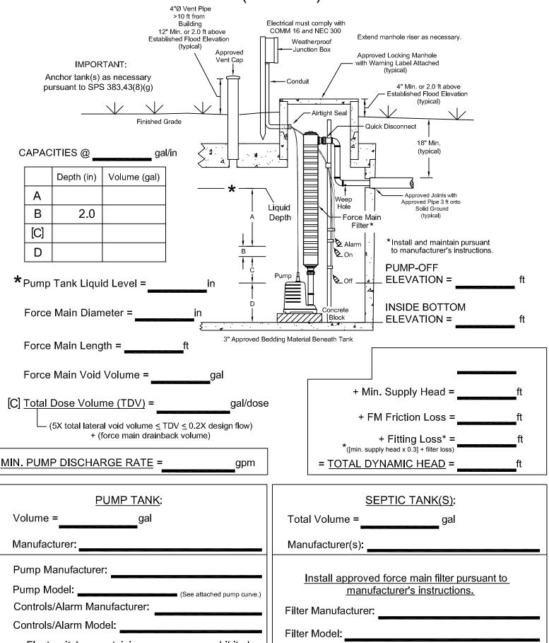
Float switches containing mercury are prohibited.
