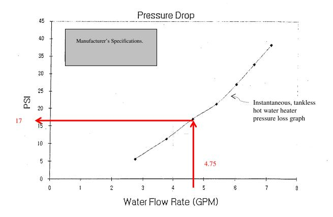
Figure 33 is a Pressure Loss Graph for the two instantaneous tankless hot water heaters and provided with the manufacturer's specifications.
