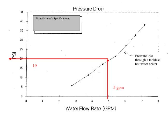
WSFU's downstream of the tankless, instantaneous hot water heater; 6 wsfu's. Convert to GPM using Table 382.40-3; 5 gpm..
