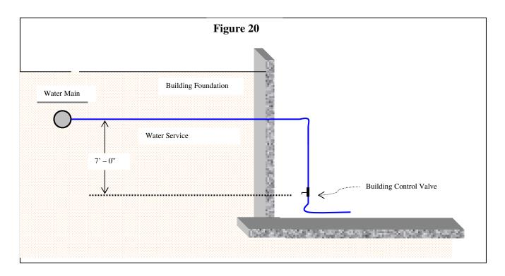
One more example: You have been contacted to install the water service piping from a water main installed at an elevation of 103 feet to a slab constructed building with a building control valve at an elevation of 117 feet. The building control valve is higher in elevation than the water service is. There will be a pressure loss through the water service piping due to this elevation difference.
